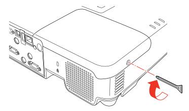
**Note:** Be sure the lamp cover is securely installed or the lamp will not come on.
